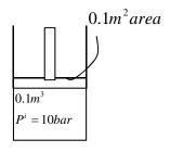
Now we need to determine  $\underline{W}$ s. The work done by the gas (subscript g) and the atmosphere (subscript a) will be equal to the work done on the piston. The gas and atmosphere are closed systems that change size.
